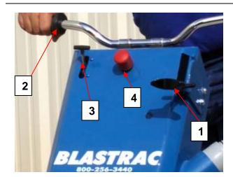
The grinding machine must be lifted by pushing down on the handgrip (2) and pulling back on the operating lever (1). Pulling back on the operating lever (1) will lower the support and take the weight off the grinding disc. Pull throttle (3) all the way back or push Estop (4).
