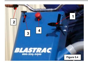
The grinding machine must be lifted by pushing down on the handgrip (2) and pulling back on the operating lever (1). Pulling back on the operating lever (1) will lower the kick stand and take the weight off the grinding disc. Pull throttle (3) all the way back or push Estop (4).
